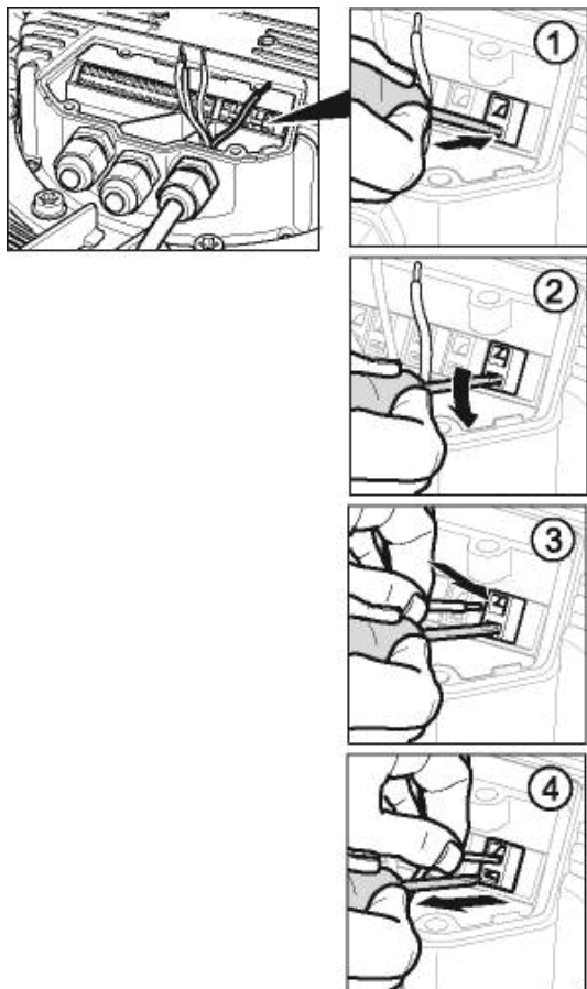
Fig. 2: Connecting wires to terminals
